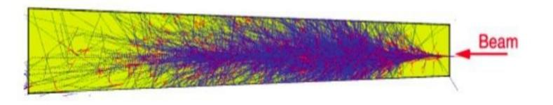
Entire shower passes active medium Active medium = absorber medium Typically inorganic crystals with high photon yield with N<sub>photon</sub> (t) ~ E  $\Rightarrow \sigma(E) \sim \sqrt{E}$
